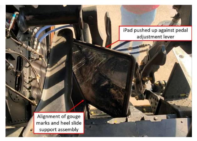
NTSB investigators were able to align gouge marks on the accident flight crew's iPad with a sharp, vertical metal piece of the co-pilot's heel slide support assembly. NTSB Photo
