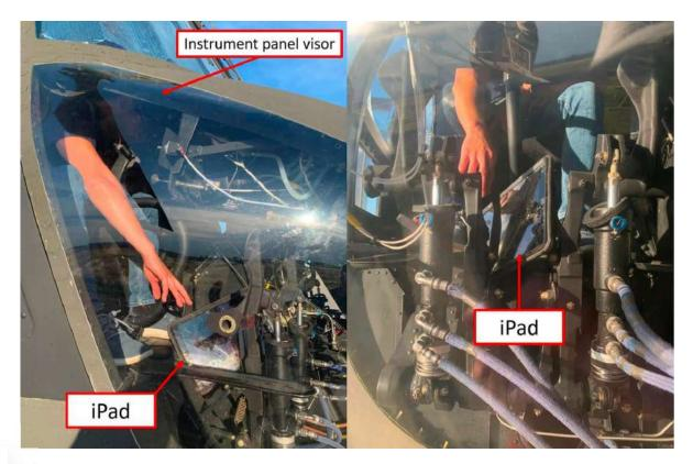
Investigators demonstrated how seat restraints and the instrument panel visor would have prevented the co-pilot from quickly retrieving the jammed iPad. NTSB Photo
